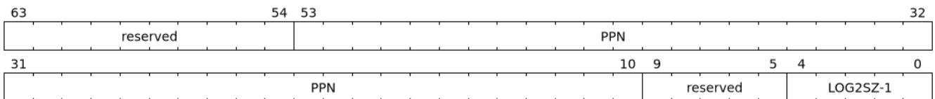
Figure 44. Page-Request-queue base register fields
